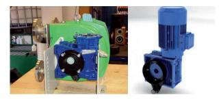
Contrary to the most gearboxes installed for this kind of application, the worm gear reducer offers the following advantages:
